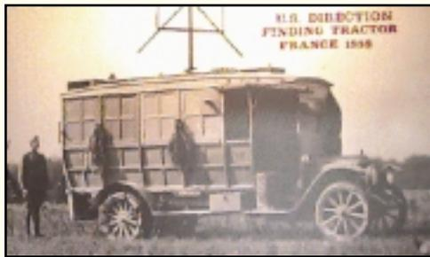
During the early 1900s, the Army operated from mobile as well as fixed installations. The museum displays a picture of a mobile U.S. direction finding truck, or “tractor” in the terminology of the time. The truck had a DF antenna, which was turned by hand from the inside. By measuring the angle of entry and the skip of a signal coming in and bouncing off the ionosphere,
